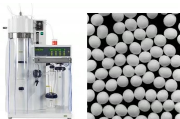
Fig. 1 (Left) Spray-dryer. (Right) Particles after spray-drying. Figures are taken from Buchi Webinar.
