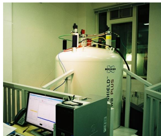
Fig. 2 Bruker AvanceIII: One of solid-state NMR magnets in Grey group. http://www.ch.cam.ac.uk/group/grey/lab-facilities
