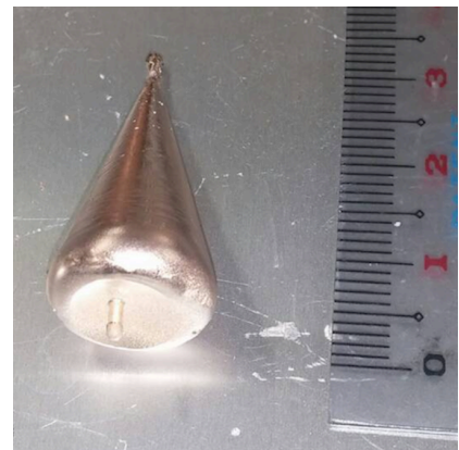
Figure: Brazing material suitable for ceramics/metal joining found in this research.
