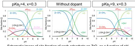
Schematic image of site fraction of each adsorbate on  $ZrO_2$  as a function of pH
