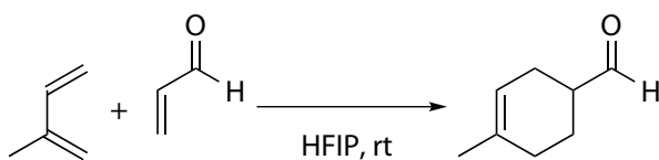
Fig. 4 Diels-Alder reaction using isoprene and acrolein.
